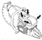
Check the air filter and replace if necessary.
